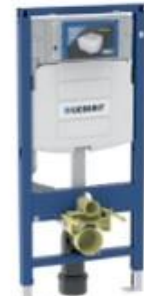
Geberit Duofix Geberit Duofix element for wall-hung WC, 112 cm, with Sigma concealed cistern 12 cm and Power & Connect box 111.900.00.5
