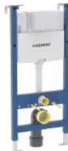
Geberit Duofix Geberit Duofix element for wall-hung WC, 112 cm, with Alpha concealed cistern 12 cm, 4.5 / 3 litres 224.095.00.1
